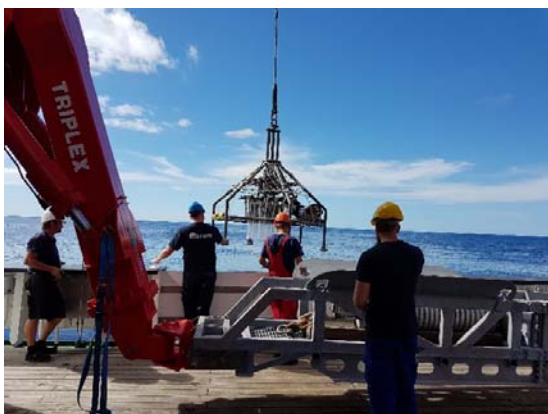
Deployment of the multiple corer with the video telemetry system (left) and a snapshot of the sampling technique on Gloria Knolls (GeoB22222-2).
