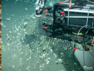
Fig 2: Pushcore sampling in front of the benthic chamber on a field of living vesicomyids.
