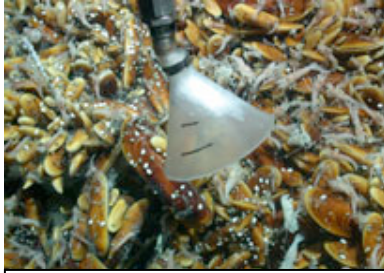
Fig 1: Sampling gas bubbles from a mussel bed (DIAPIR site; All Photo sources: MARUM)
