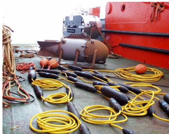
DeepTow Streamer and Sidescan with 2 tons depressor weight
