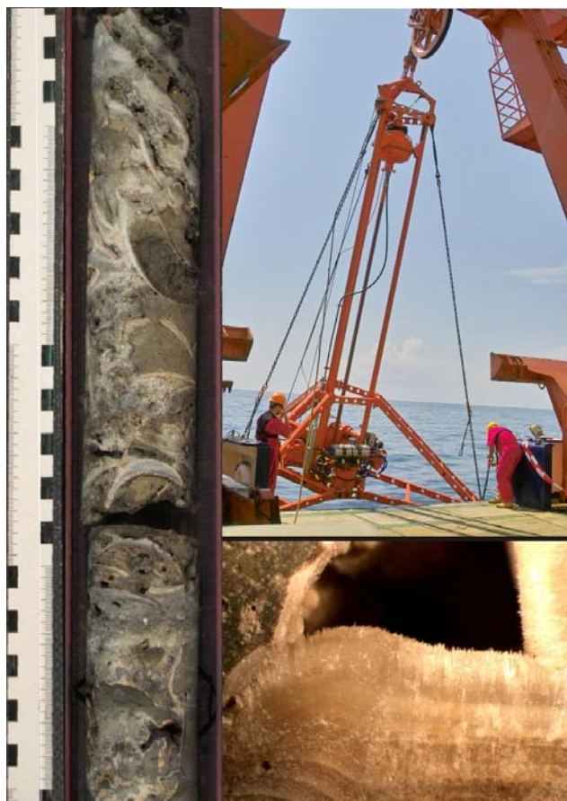
Figure 1: Deployment of the BGS Rockdrill system on METEOR 66/3a, Core M66-129-Mound Iguana (left), calcitic filling (below)
