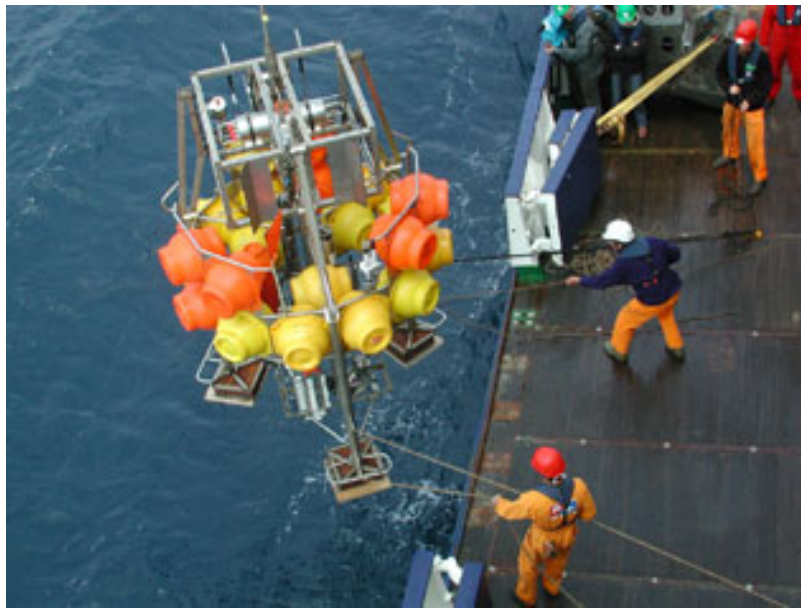
Figure 4: Deployment of a GEOMAR BC-Lander carrying an OceanLab bioluminescence observatory.
