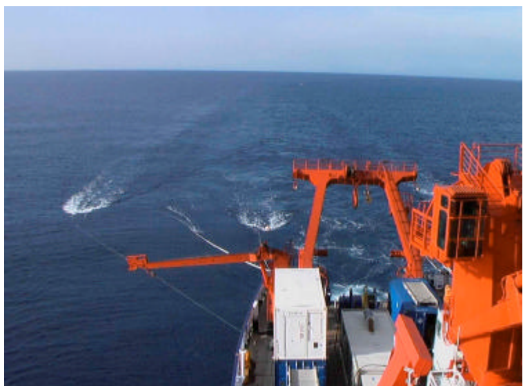
Figure 5: Towing of shear boards for seismic sources.
