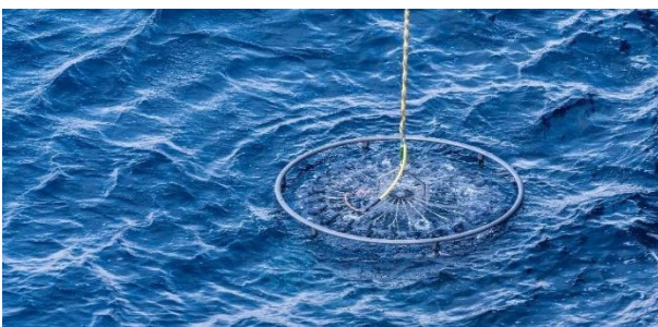
Figure 2 Deployment of titanium CTD frame. (Photo: C. Rohleder)
