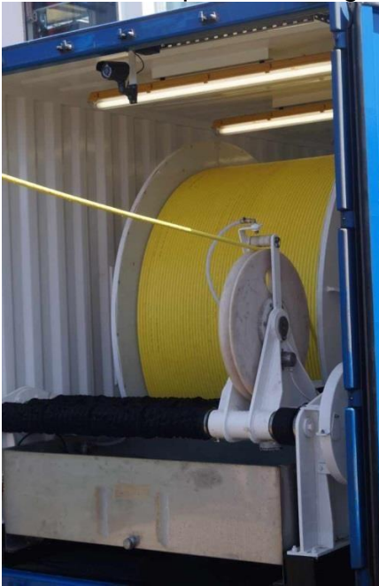
Figure 1 Winch with Kevlar conducting wire (Photo: E. Achterberg)
