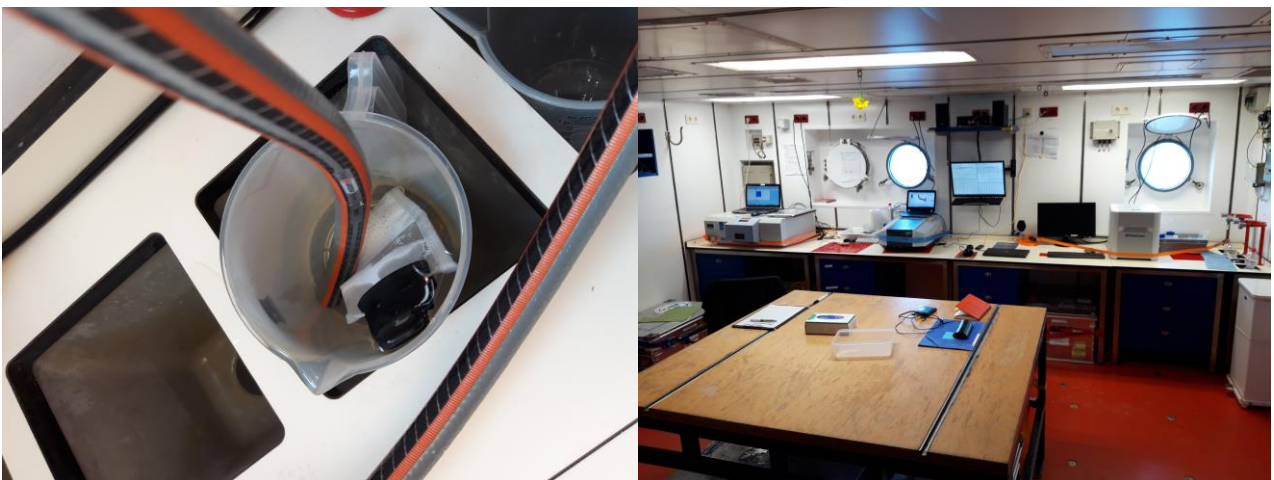
Fig. 2: Laboratory measurements. Left: SPATT-sampling for phycotoxins. Right: Fluorometer, photometer, and FlowCam (from left to right).
