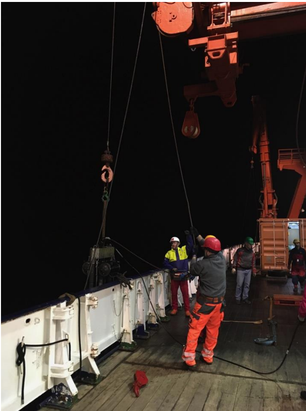
After sampling of the sea floor the vibracorer returns on board RV METEOR
