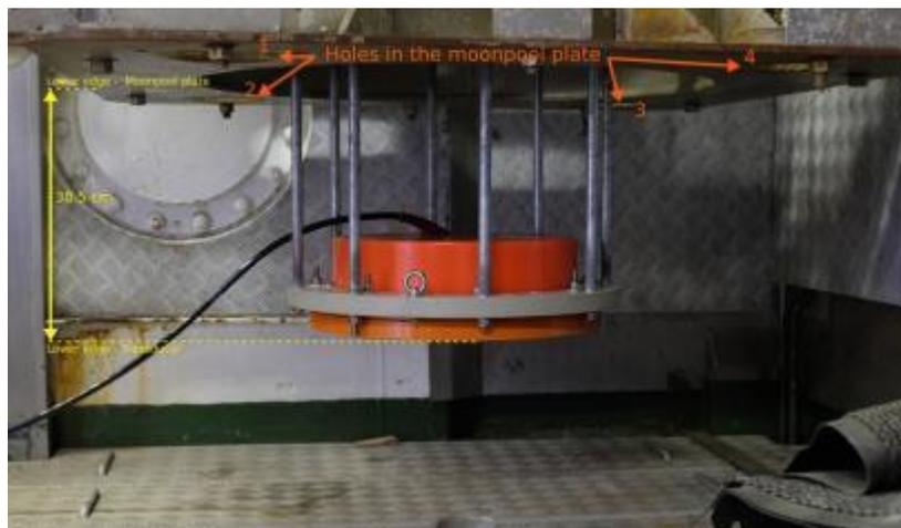
**Figure 2:** ES38-7(orange) attached to the moonpool plate with 50 cm long spacer elements.
