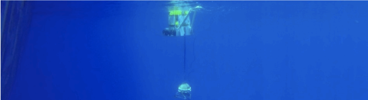
French OBS RR40 seconds before being pulled out of the water. Hooked by the ship crane, this type of instrument swings like a double pendulum, and also needs to be approached carefully due to its protruding parts.
