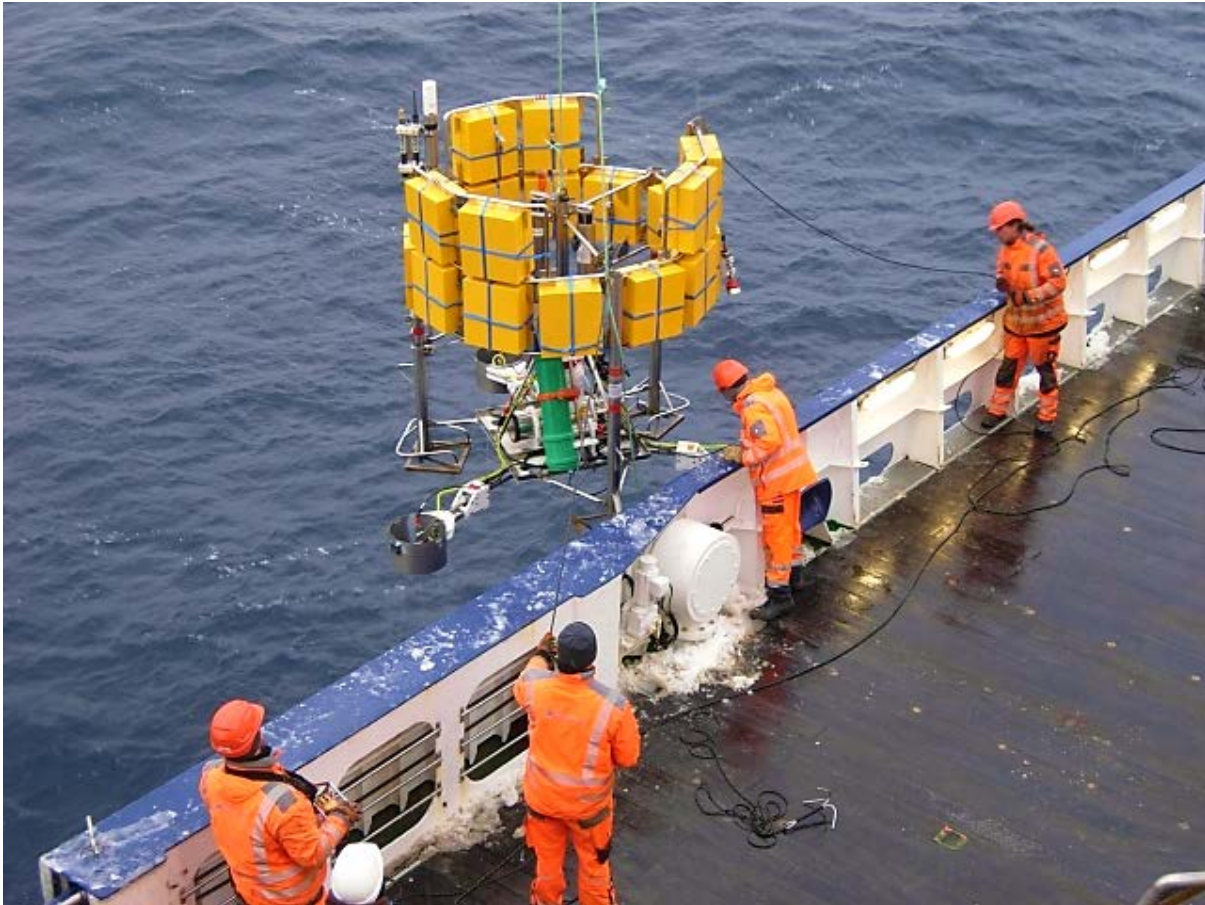
Fig. 1: Recovery of the “arcFOCE” (arctic Free Ocean Carbon Enrichment) system after its first test deployment west off Svalbard.
