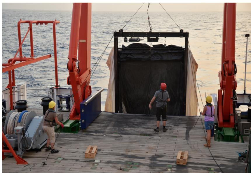
**Fig. 2** Deployment of the 10m<sup>2</sup>-MOCNESS
