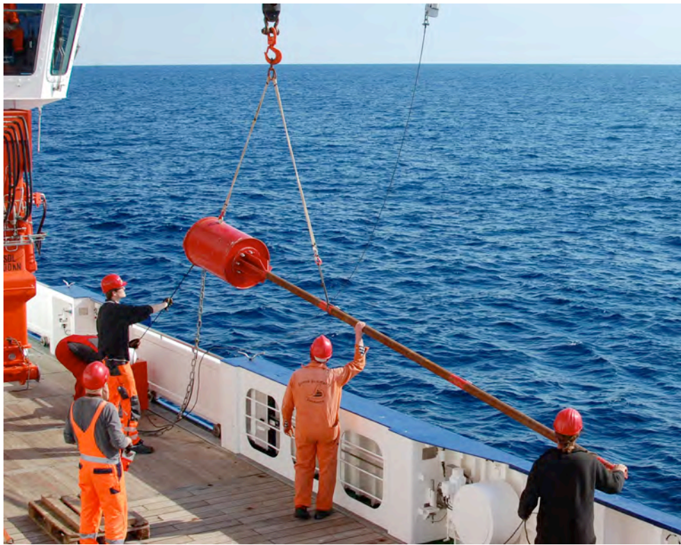
Fig. 1: Deployment of the temperature lance.
