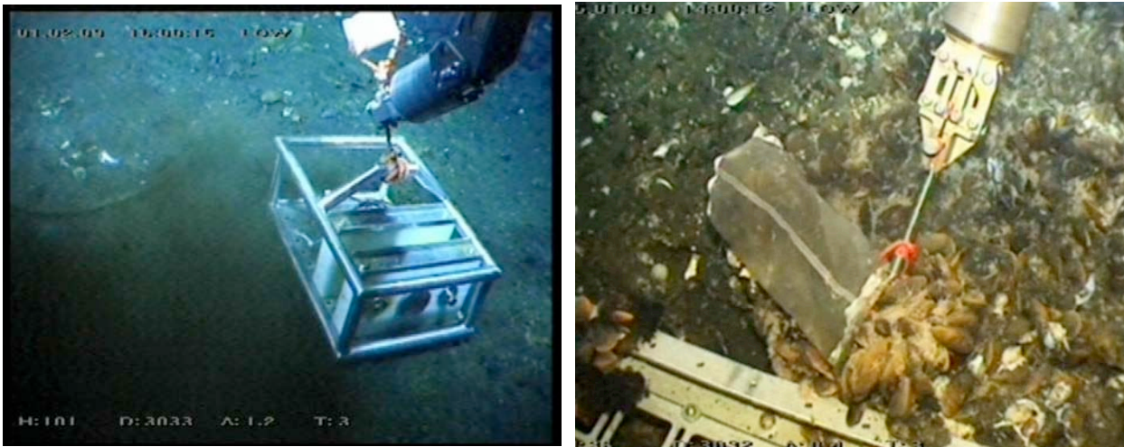
Fig. 3: Images from our ROV dive at the Logatchev hydrothermal vent field. On the left, the recovery of the OBP and on the right, the sampling of Bathymodiolus mussels near the active vent site Irina II. Copyright: IFM-Geomar
