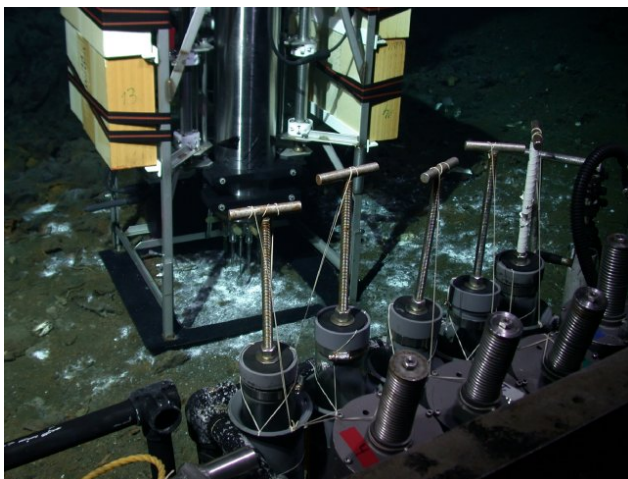
Fig. 3: Positioning of the profiler on a microbial mat.
