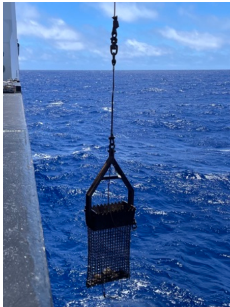
Fig. 1: A chain-bag dredge is being pulled back onto the deck of R/V SONNE (Photo: H. von Drenkmann)
