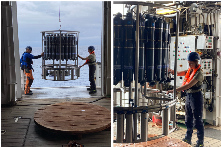
Fig. 1a, b: Retrieving the CTD. Left panel: The crew (left) and the scientific team (right) work hand in hand (Photo: J.G.).
