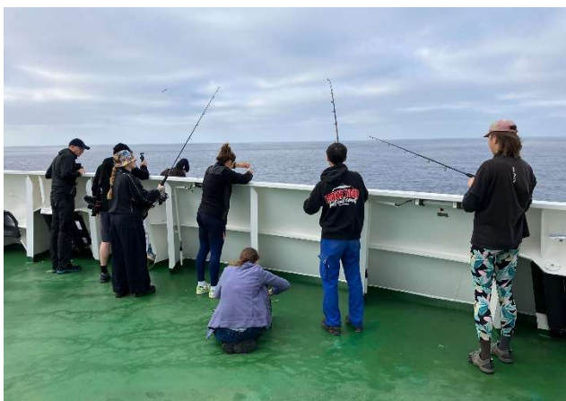
Figure 1: Using three fishing rods and precisely calculated line lengths, the members of the hydro-acoustics group manage to position the calibration sphere beneath the ship, exactly within the sound cone of the 18 kHz transducer. (@ Gerhard Bohrmann)
