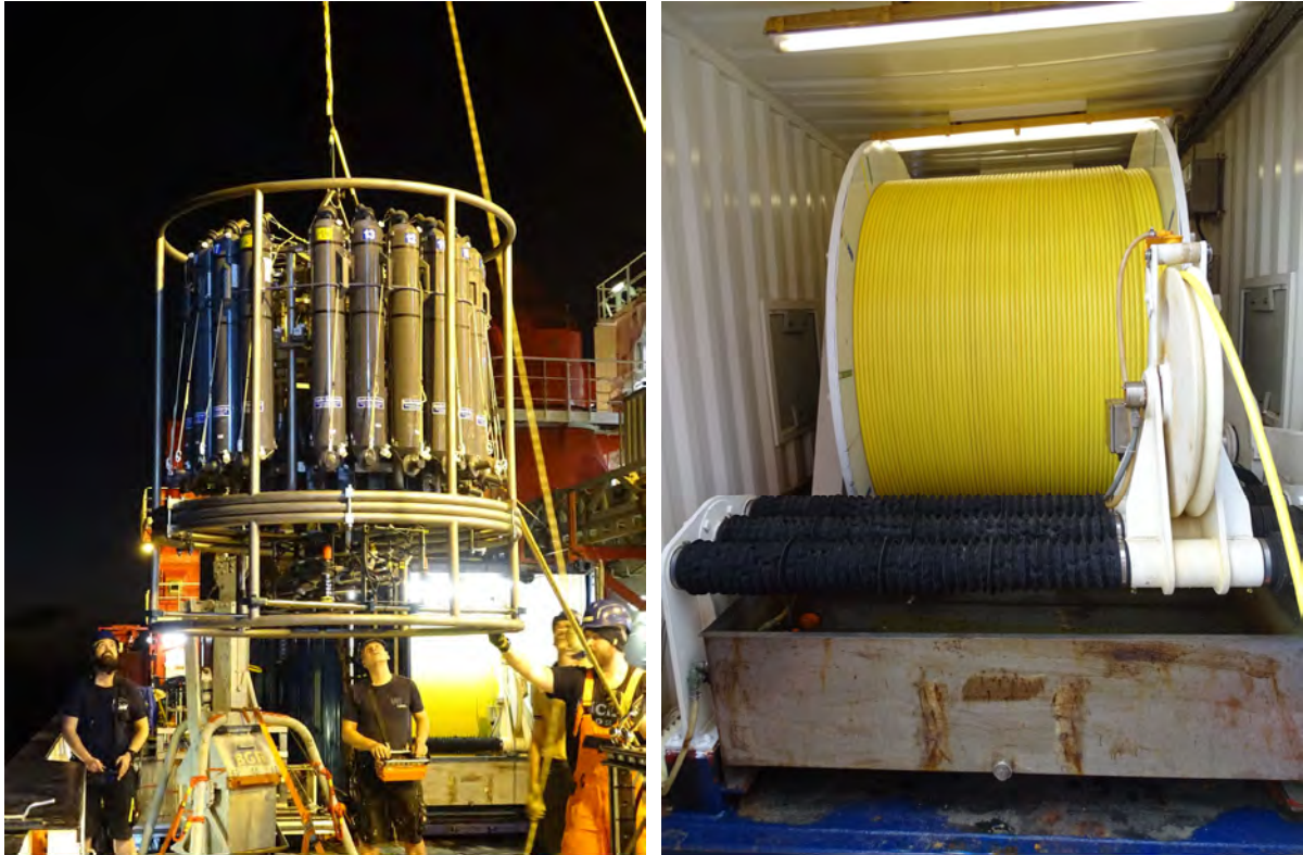
GEOMAR's ultra-clean trace metal CTD-Rosette is deployed over the starboard side of RV SONNE (left). It is operated on its own 7000-m-long metal-free cable/winch (right) using the ship's crane. Photos: Simone Sturm.
