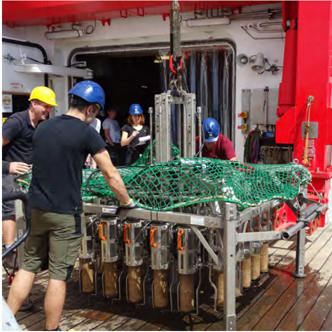
Left: A video-supported 20-core multicorer brings short sediment cores from the seafloor to the deck of the vessel (photo: Simone Sturm). Right: Laboratory technician René Herbst processes geochemical samples from the multicorer in the cold lab (photo: Robert Sommerfeldt).
