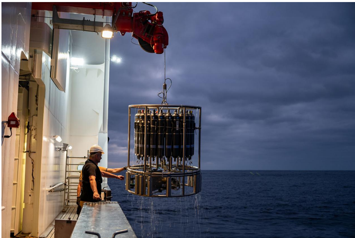
CTD probe with rosette sampler being heaved on deck after successful deployment (picture: V. Diekamp).
