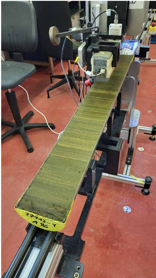
Left: Documentation of a sediment core with a multi-scanner core logger. Right: A gravity corer with a sediment core being heaved on deck (pictures: P. Grunert).
