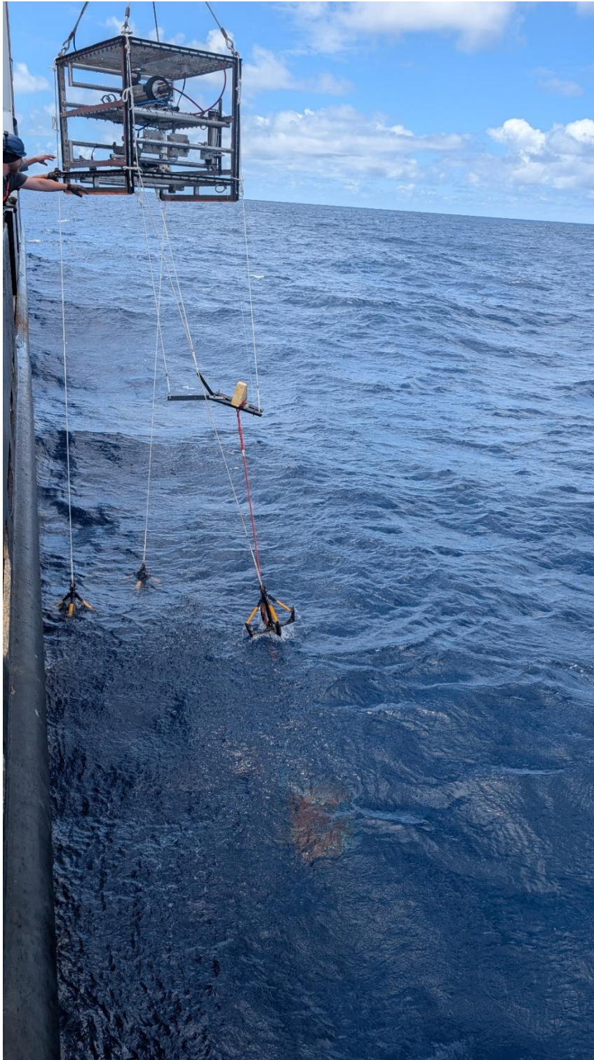
Fig. 1: Recovery of the red OBS that could not be released (immediately below the surface) below the camera sledge OFOS. Below the OFOS the three grapnels and the Y-shaped frame are visible, with which the OBS could finally be captured at its yellow float in 3000 m water depth.
