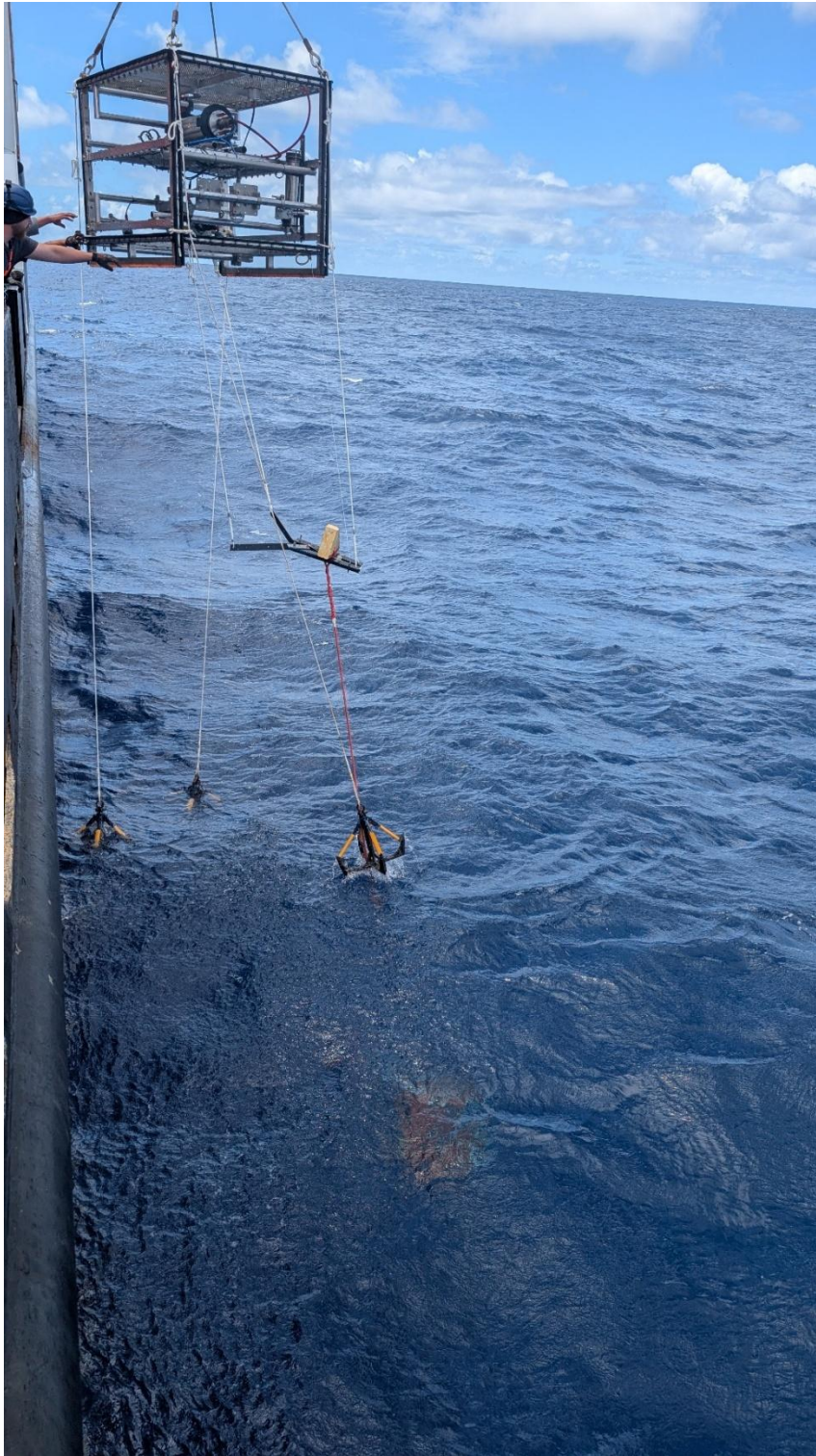
Fig. 1: Recovery of the red OBS that could not be released (immediately below the surface) below the camera sledge OFOS. Below the OFOS the three grappels and the Y-shaped frame are visible, with which the OBS could finally be captured at its yellow float in 3000 m water depth.
