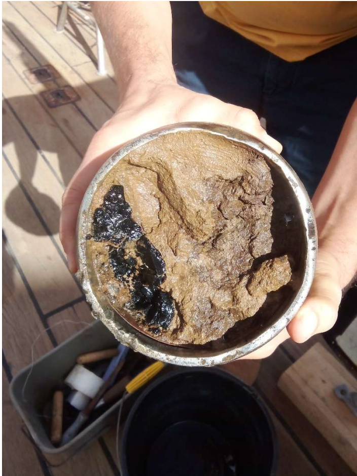
Fig. 3: Sediment core containing a large basaltic glass fragment in the Core Catcher, which proved that the core pierced the sediment cover completely and reached the basaltic oceanic crust.
