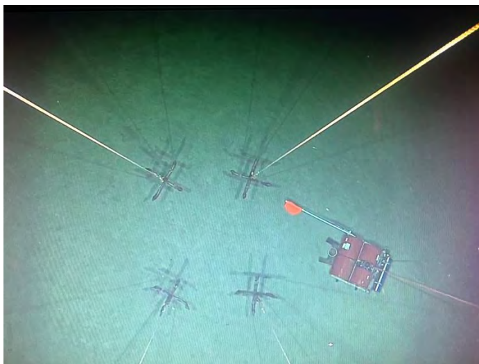
Fig. 2: View of the four grappels underneath the camera sledge OFOS, which were used for the recovery of the OBS that could not be released (to the right of the picture).
