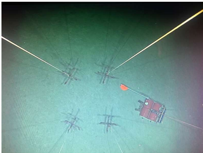
Fig. 2: View of the four grapples underneath the camera sledge OFOS, which were used for the recovery of the OBS that could not be released (to the right of the picture).
