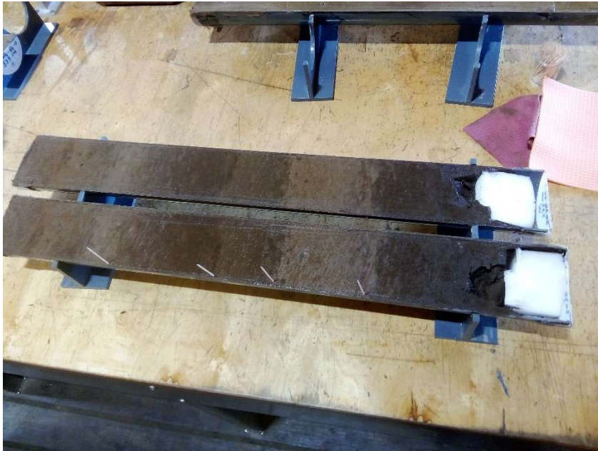
Fig. 2: One meter long section of a sediment core cut into two halves. The core recorded the direct transition between the basaltic crust and the sediments (the white foam prevents slipping of the sediments in the liners).
