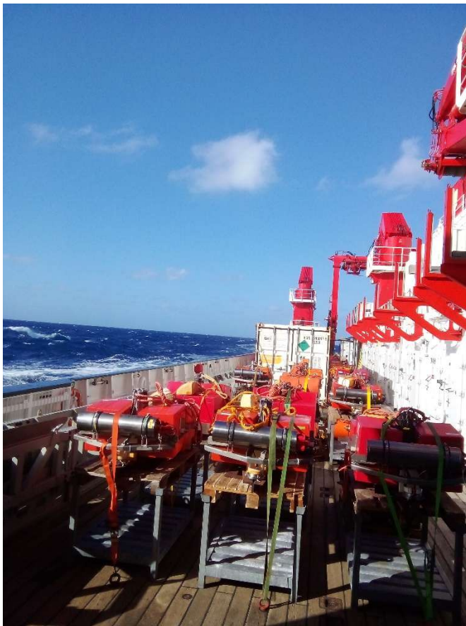
Abb. 2: Ocean Bottom Seismometers ready for deployment on the working deck.
