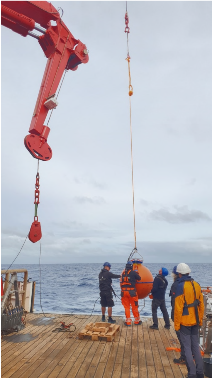
Figure 1: Recovery of the top-buoy of mooring LR2 over the rear A-frame of RV Sonne. The buoy consists of the spherical orange flotation device, with an Acoustic Doppler Current Profiler (ADCP) mounted inside the sphere. Photo: J.Mette.
