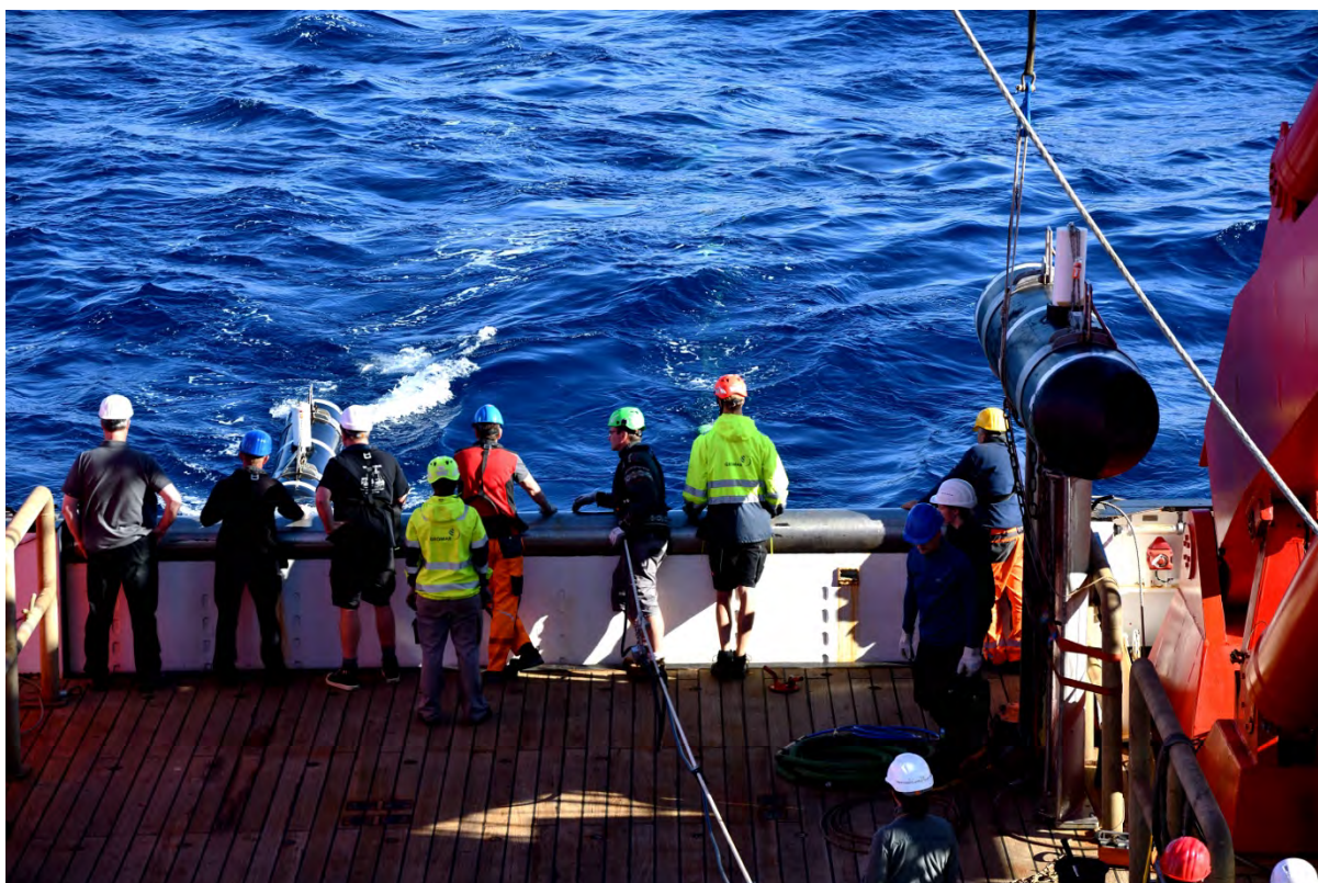
Figure 2: Deployment of the 3D seismic system with the port side paravane in the water and the starboard paravane still on deck. Photograph: Aude Lavayssiere.
