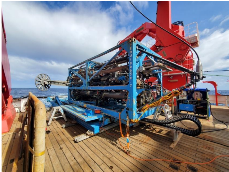
Fig. 2: The MeBo200 marine drilling rig is being prepared for its first deployment. Photo: Fabian Hampel
