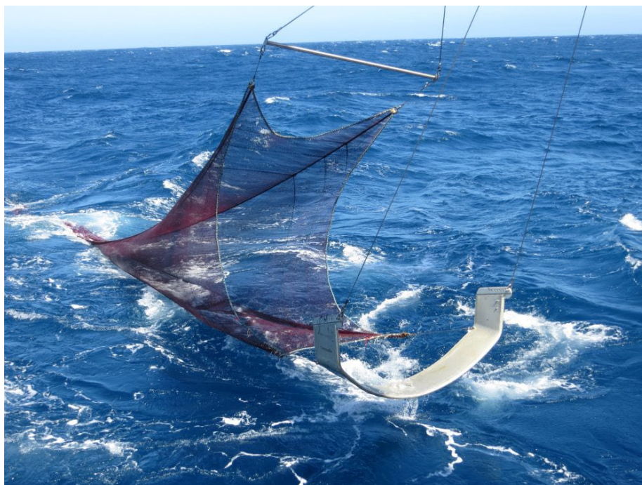
Fig. 3: First deployment of the Isaacs-Kidd Midwater Trawl. Photo: H. Auel
