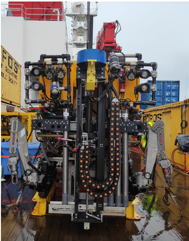
Figure 1: ROV ROPOS with the drill tool ROCS mounted at the front side (left; photo: T. Kuhn) and a drill core from the AURORA field in Cluster 12 (photo: S. Sturm).
