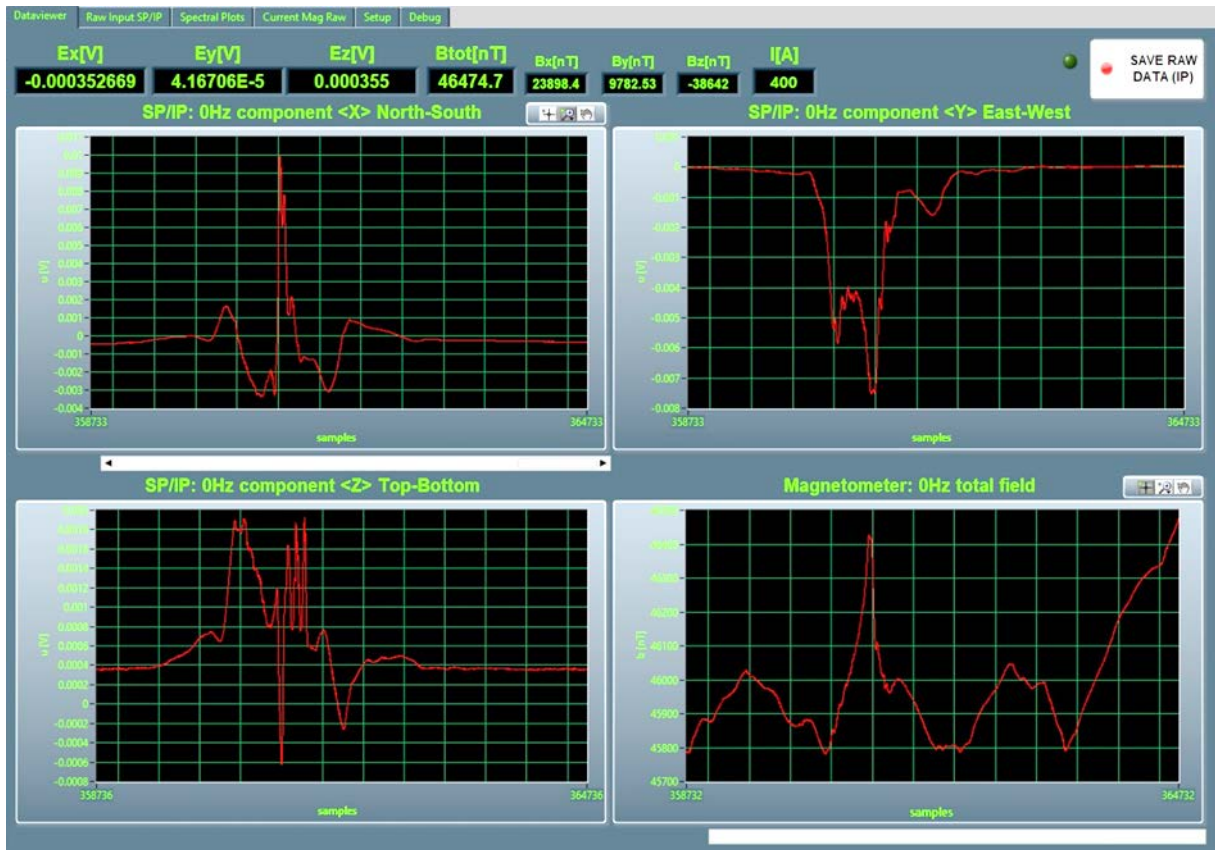
Data example of a self potential anomaly in three components and magnetic anomaly over massive sulphides in the inactive region of the KAIMANA field.
