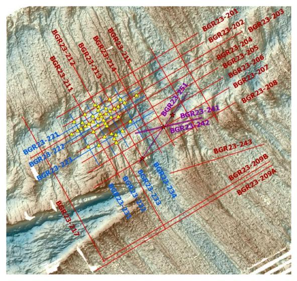
Working area around the Rodriguez Triple Junction: Regional profiles (red), additional profiles at the OCC (blue) and at the Kairei hydrothermal field (KHF) (purple). Measured profiles are annotated with profile names. During the two-week profiling, 41 ocean bottom seismometers (OBS) at the OCC (yellow triangles) and 5 broadband OBS at the KHF recorded all airgun shots while the shot spacing was increased to 60 seconds during turns for profile change.
