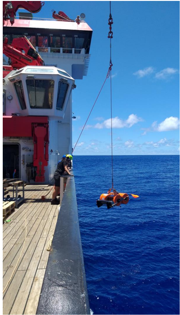
Deployment (left) and recovery (right) of ocean bottom seismometers (Foto: Martin Engels)
