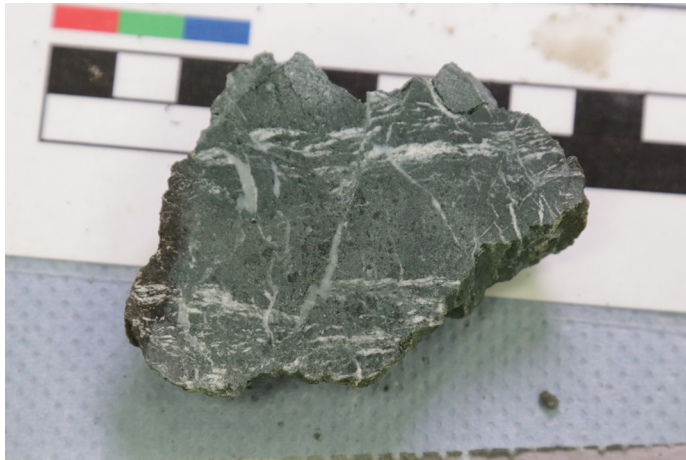
Low-grade metamorphic volcanic rock with veinlets formed by tectonic deformation. Foto: SO299 Science Party.
