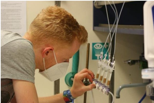
Figure 2: Acidified, filtrated seawater is running over columns for extraction of DOM (Photo: H. Frazao).
