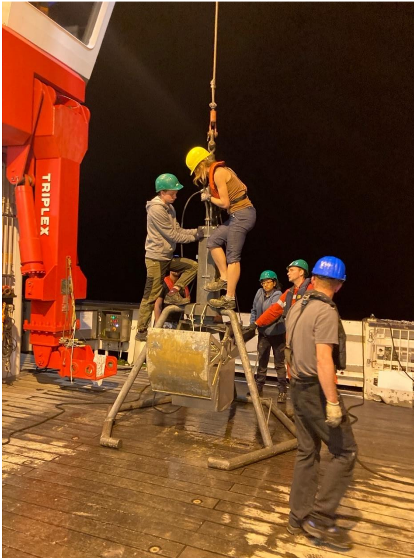
Fig. 5 The box corer is prepared for deployment.
