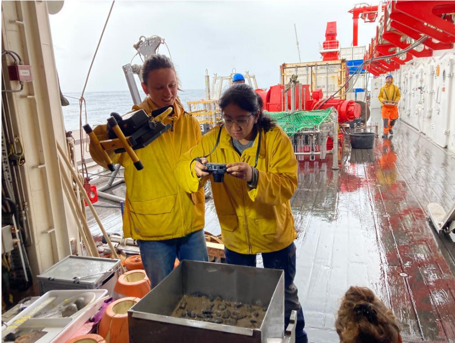
Fig. 3: Documenting the nodule coverage with the boxcorer
