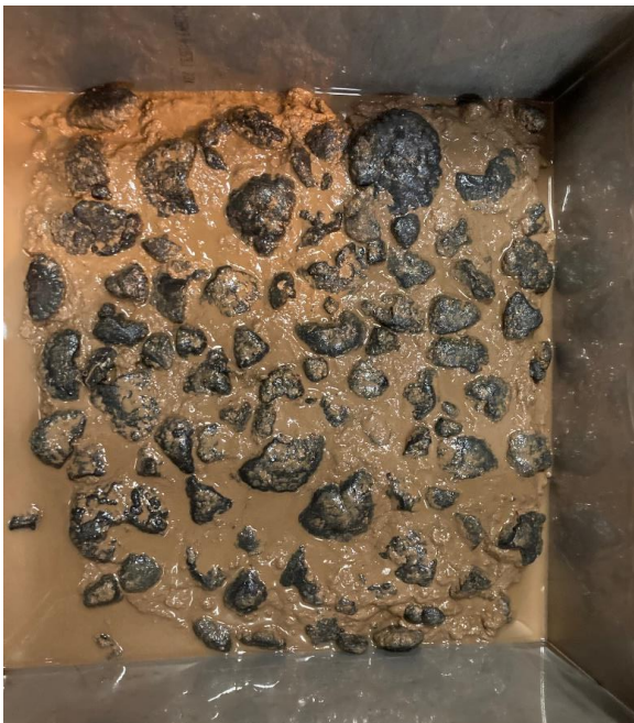
Fig. 3: Box corer with manganese nodules.
