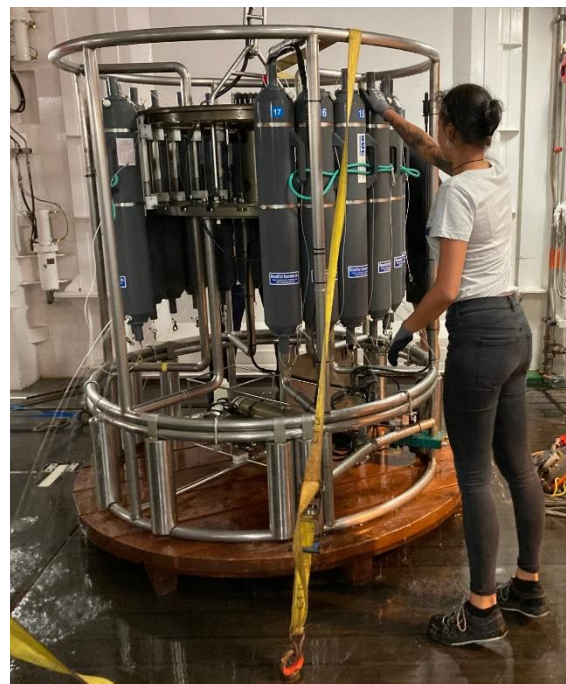
Fig. 2: CTD on deck after successful sampling.
