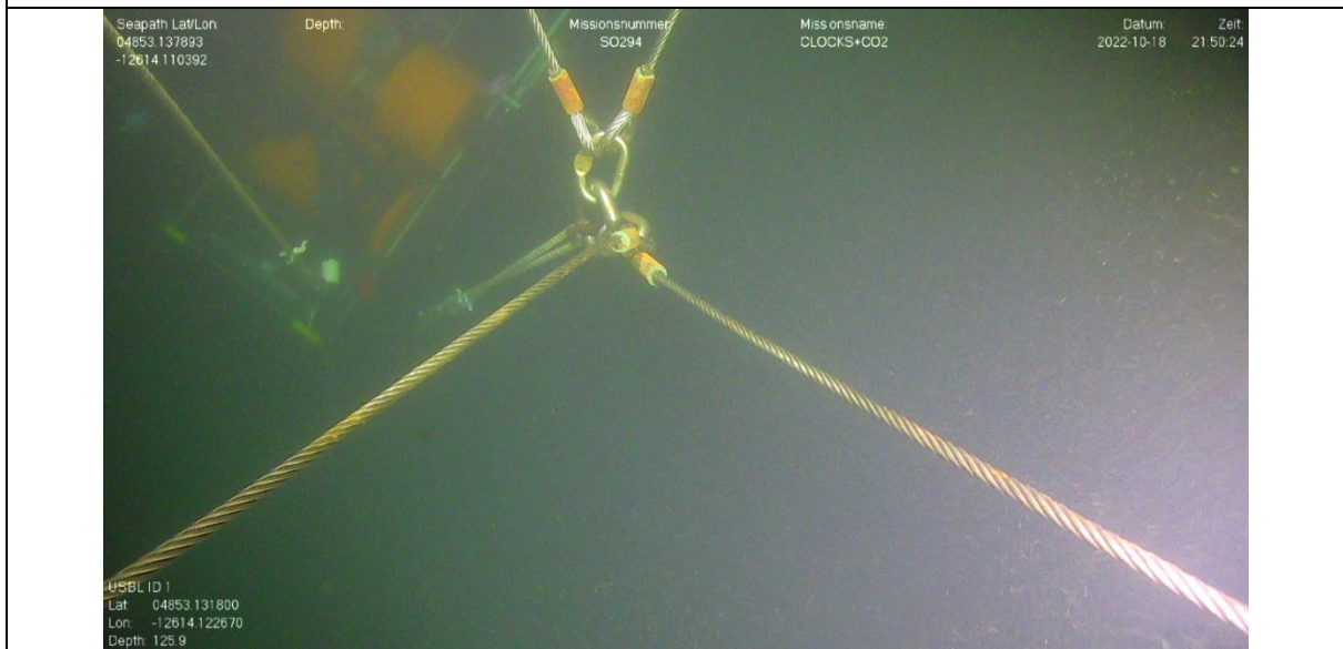
(b) Only four minutes later, the MT instrument came into sight again and the winchman successfully connected the hooks to the instrument's own frame and one of the electrode-arms. He then immediately heaved OFOS and thus pulled the MT station from the bottom.
