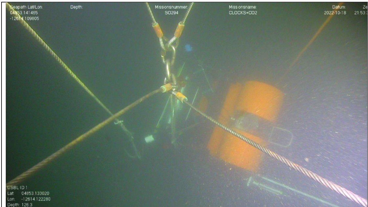
(c) The OBMT came free of the seafloor and anchor and floated quicker to the sea surface. We were then able to retrieve OFOS.
