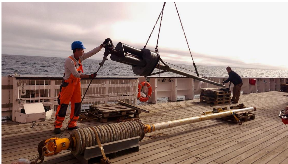
Figure 4: Deployment of the heat-probe (Photo: Sarah-Marie Kröger).
