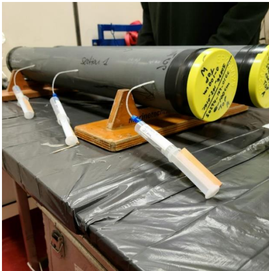
Figure 6: Photograph taken during sampling of the core segments with rhizones in the laboratory onboard SONNE (Photo: Sarah-Marie Kröger, Univ. Kiel)
