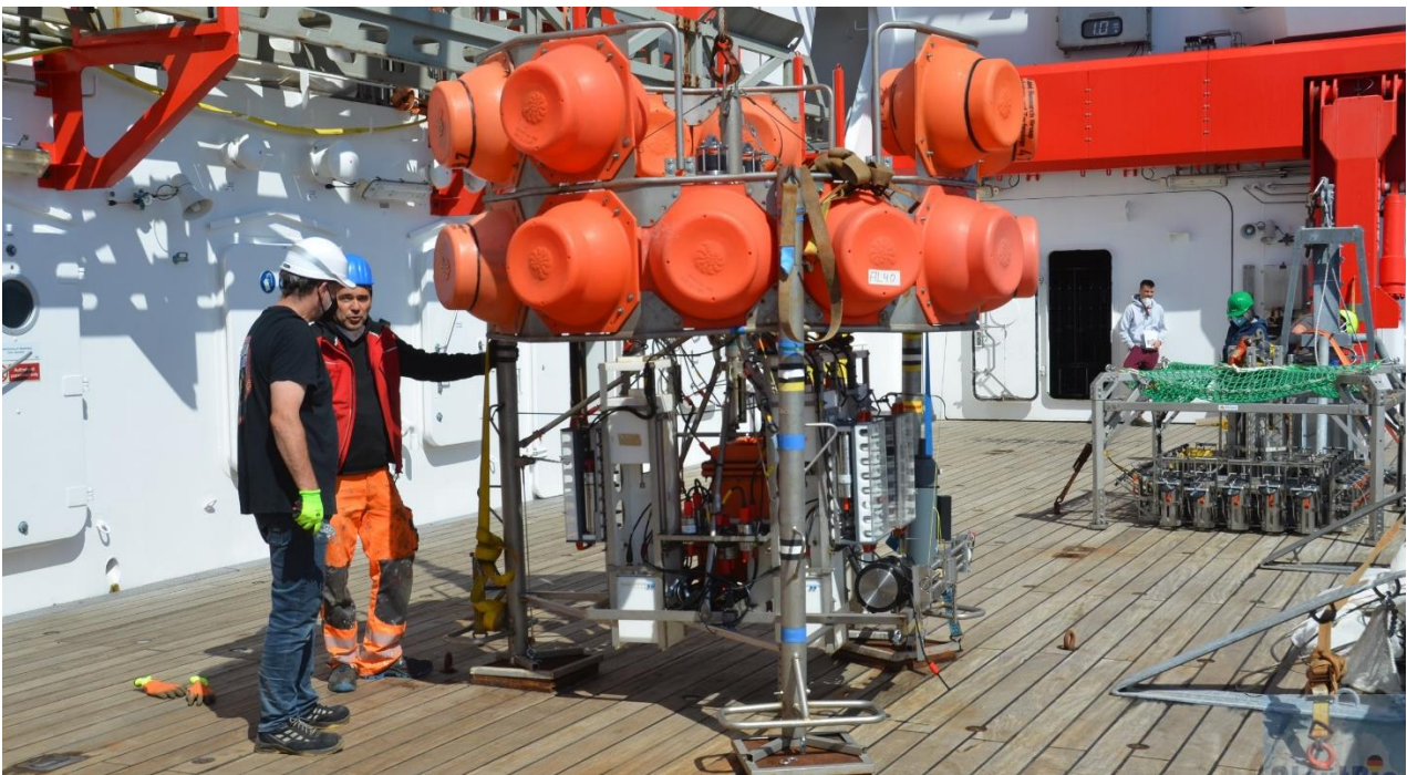
Figure 5: Freefall lander system on board FS Sonne before deployment.
