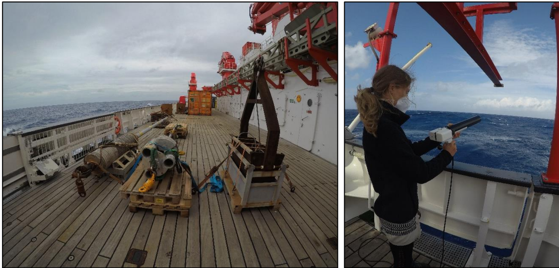
Figure 2: i) all the instruments to be deployed assembled on deck of the R/V Sonne, and ii) Mona Lütjens shooting an XSV probe to measure the water column sound velocity.
