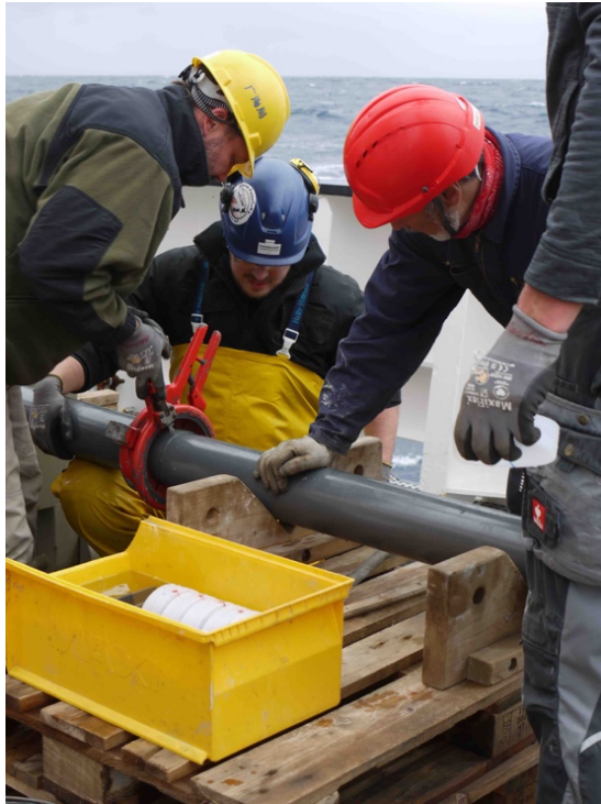
Pictures 1-2: Left: The coring team cutting a long sediment core into 1 m sections. Right: Initial collection of sediment samples from a long sediment core (photos: SO290, K.Pahnke, CC BY 4.0)
