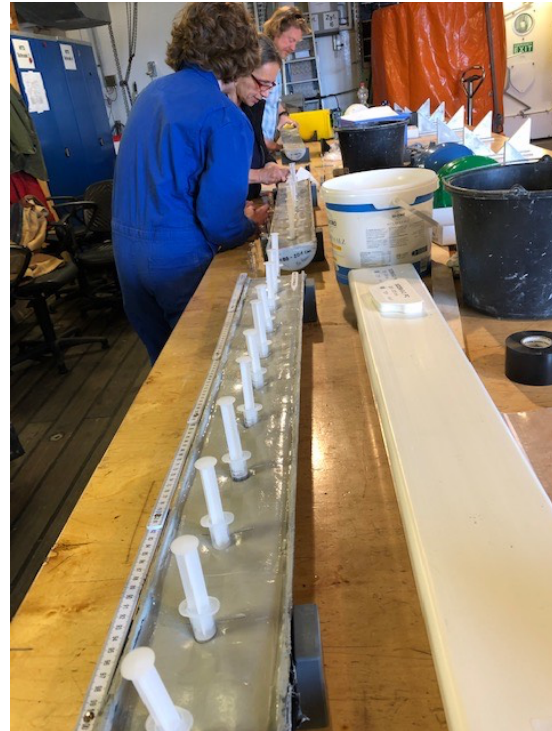
Pictures 1-2: Left: The coring team cutting a long sediment core into 1 m sections. Right: Initial collection of sediment samples from a long sediment core (photos: SO290, K.Pahnke, CC BY 4.0)
