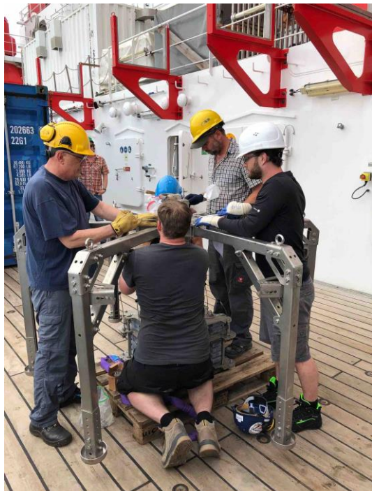
Fig. 2: Assembly of the multi-corer (SO290)
