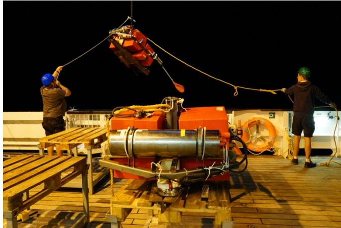
Figure 4: An ocean bottom seismometer (OBS) is launched after a short float test. OBSs record the energy generated by air pulses traveling through the oceanic crust and into the Earth's mantle. They are installed free-falling on the seafloor and can be recovered by an acoustic signal that releases the anchor. OBSs then rise independently to the water surface. The data are stored on the instrument on a data logger.
