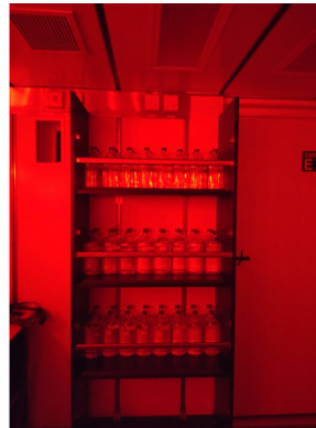
Figure 2: Incubation experiments on deep-sea organic matter degradation in the climate laboratories of SONNE at in-situ temperature (2.5 °C) and elevated temperature (6 °C). Incubations are also conducted in the dark and red light is used during sampling to inhibit algae growth.
