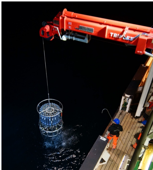
Fig. 1: CTD rosette on RV SONNE during its first deployment on SO288.
