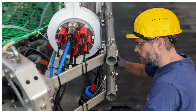
Figure 3. Alexander Kieneke (Senckenberg am Meer) checks on the OFOS camera mounted on the 20 cores Multicorer. Deployed as "TV-MUC" we were able to sample soft sediment on top of the seamount in our working area, which is geologically characterized as spreading axis west of the MAR. Foto © Viola Siegler, Senckenberg am Meer
